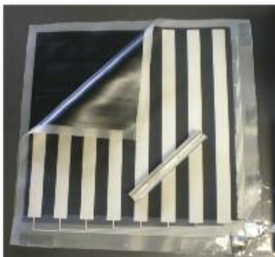
Pressure sensing pad made using flexible polyurethane film
